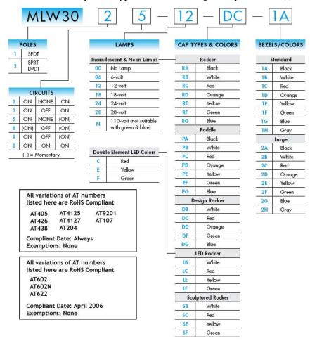
Compliant Date: All switches with date code 64 (April 2006) or later Exemptions for switch part numbers with circuits 2 and 3: None Exemptions for switch part numbers with circuits 5, 8, 9, and 0: Directive 2002/95/EC Annex #8, Cd plating on contacts
