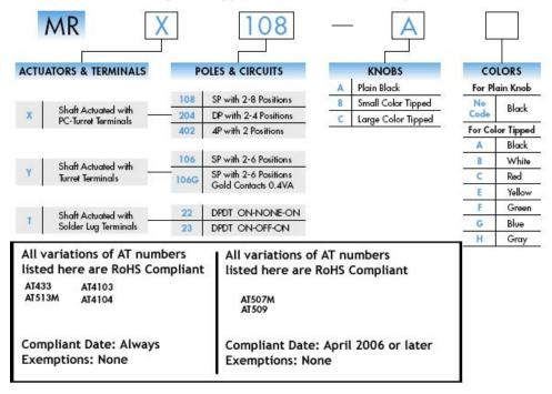
Compliant Date: All switches with date code 64 (April 2006) or later Exemptions for switches: Directive 2002/95/EC Annex #6, Pb in Cu alloy
