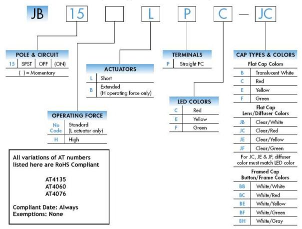
Compliant Date: All switches with date code 64 (April 2006) or later Exemptions for switches: None
